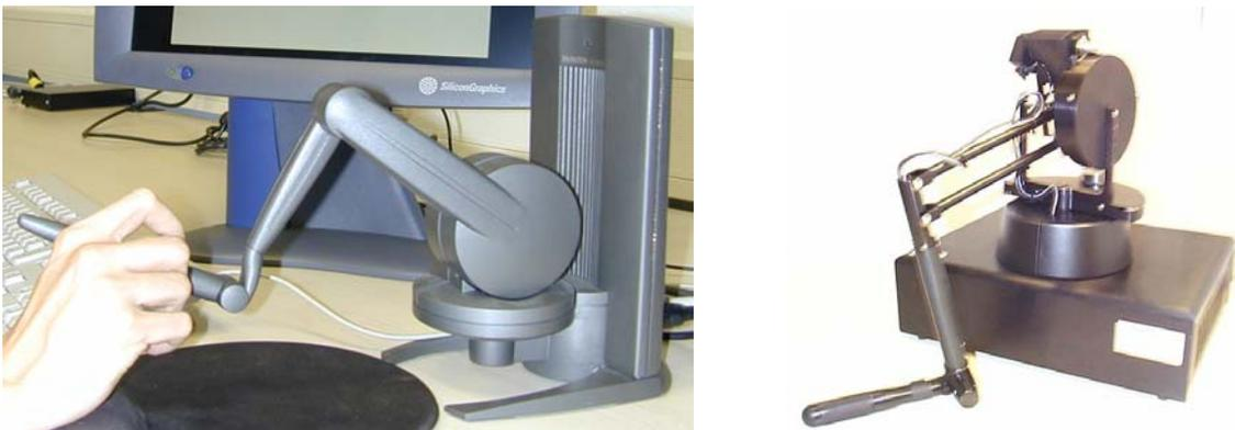
Figure 7: Phantom haptic devices with 6 degrees of freedom and 3 (left) and 6 (right) degrees of force feedback.
